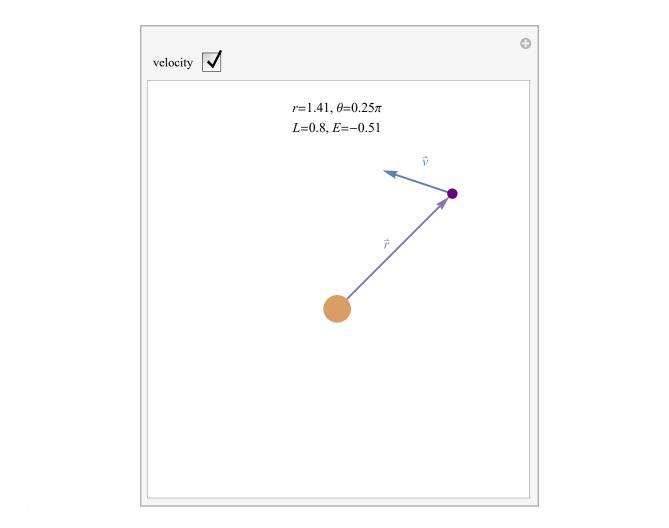
For example, if we rotate v around in a circle (but leave its magnitude unchanged), then E will be constant while L will change; L will reach its maximum value when  $\vec{v}$  is perpendicular to  $\vec{r}$  and L = 0 when  $\vec{v}$  is parallel to  $\vec{r}$ .
